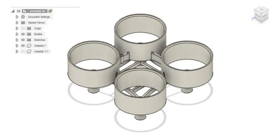
When I printed and tested this drone, it didn't have enough force to lift off the ground. After many trial and errors, my drone will now take flight. As shown below, this is my final design. The funnels are much smaller and I considerable reduced the mass.
