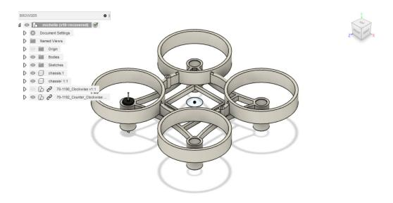
The final mass of my drone is 14.664g, while the center of mass is -1.26953mm, -0.0717751mm, 7.37933mm. The center of mass is a coordinate system (x,y,z).
